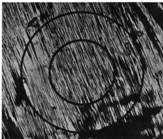
Fig. 3. Specimen 17, 5% extension. Circles show areas irradiated by large and small X-ray beams. No striae in irradiated areas. \times 50 .
